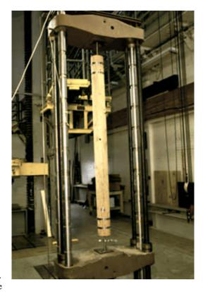
post tensioning rod. Forest Products Laboratory researchers are selecting the most promising details to develop a data base for deriving design values that will be applied in demonstration structures.
