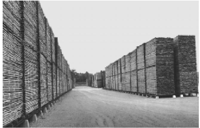
Figure 22—Well-graded and surfaced main alleys aid drainage and restrict growth of weeds.
