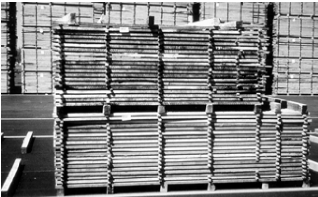
Figure 32—The protection provided by a drying shed can be seen by comparing the air-dried (on top) with the shed-dried package (bottom).
