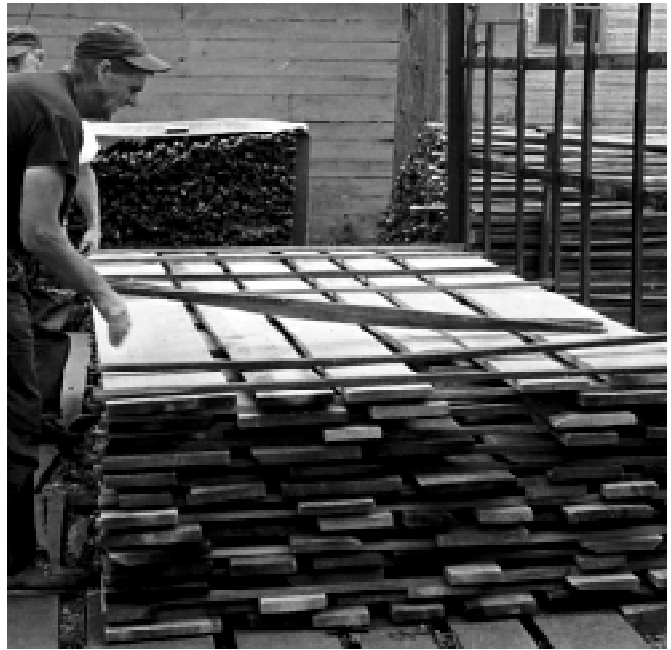
Figure 39—Sticker guides are used to improve sticker alignment.
