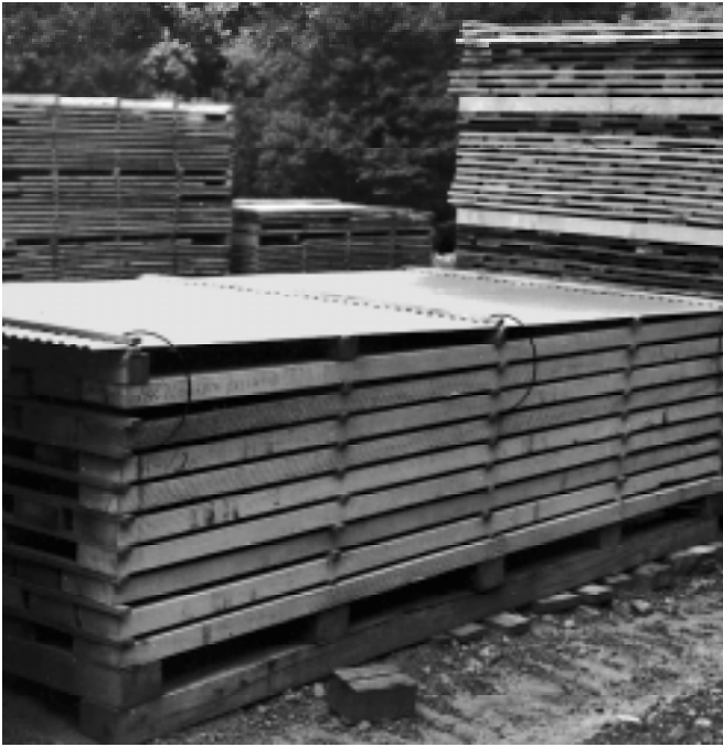
Figure 29—Loose sheets of corrugated metal are tied to the package with a “C” clamp. A sticker is laid across the top of the package on which the clamp is placed.
