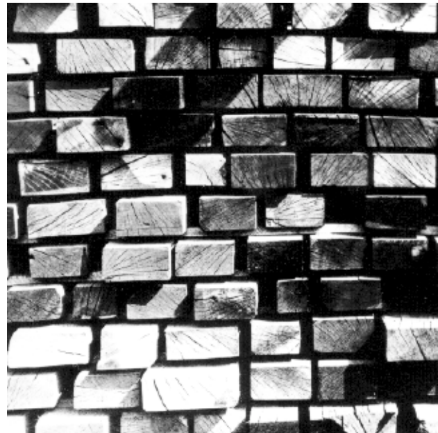
Figure 47—End checks in lumber can extend to develop splits.
