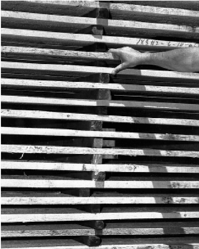
Figure 42— So that air can circulate over the board surfaces, wood stickers separate the layers or courses of lumber.
