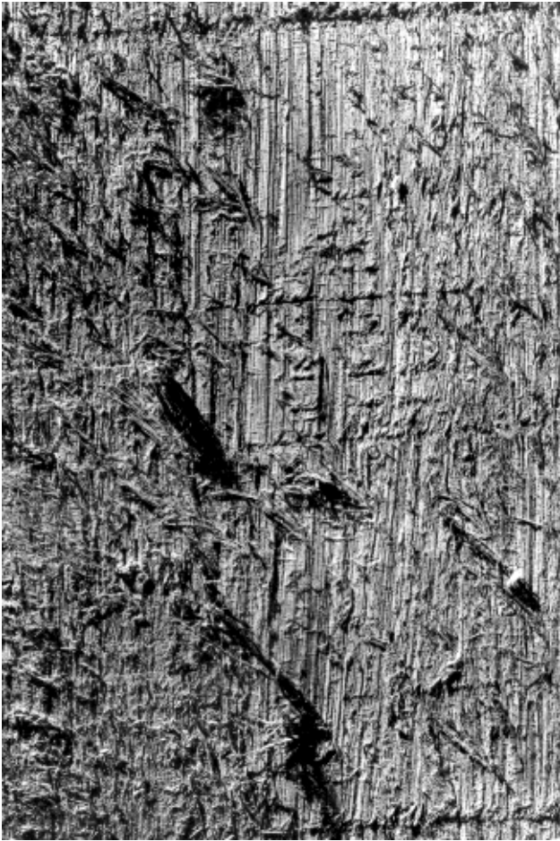
Figure 13—Area of tension wood is indicated by grain torn during machining.
