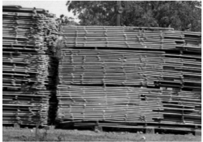
Figure 54—Example of poor sticker alignment.
