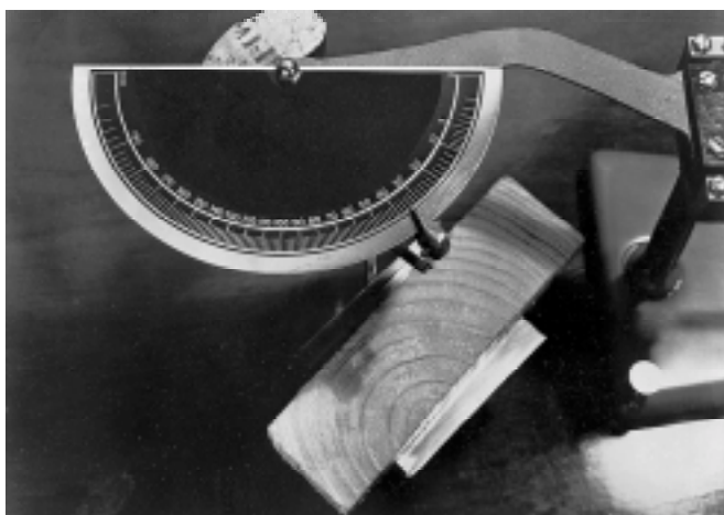
Figure 17—Self-calculating moisture content balance. The triple beam balance is provided with a special scale on the specimen pan that is used to calculate the moisture content after the section is oven-dried.
