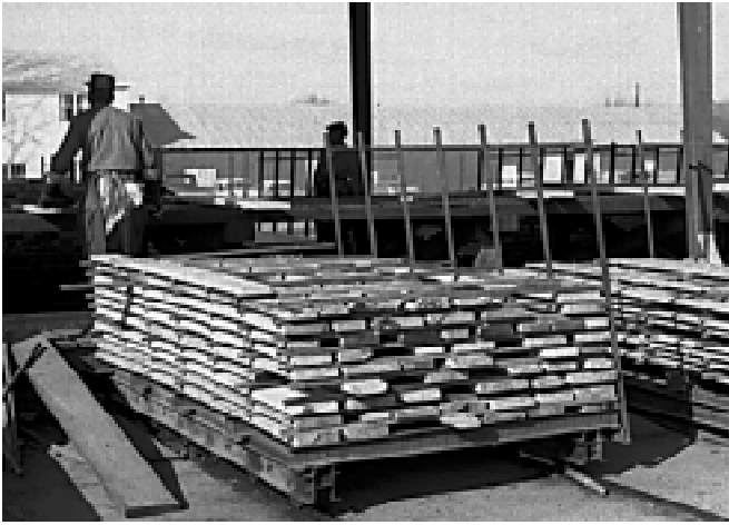
Figure 36—Lumber is sometimes manually stacked.
