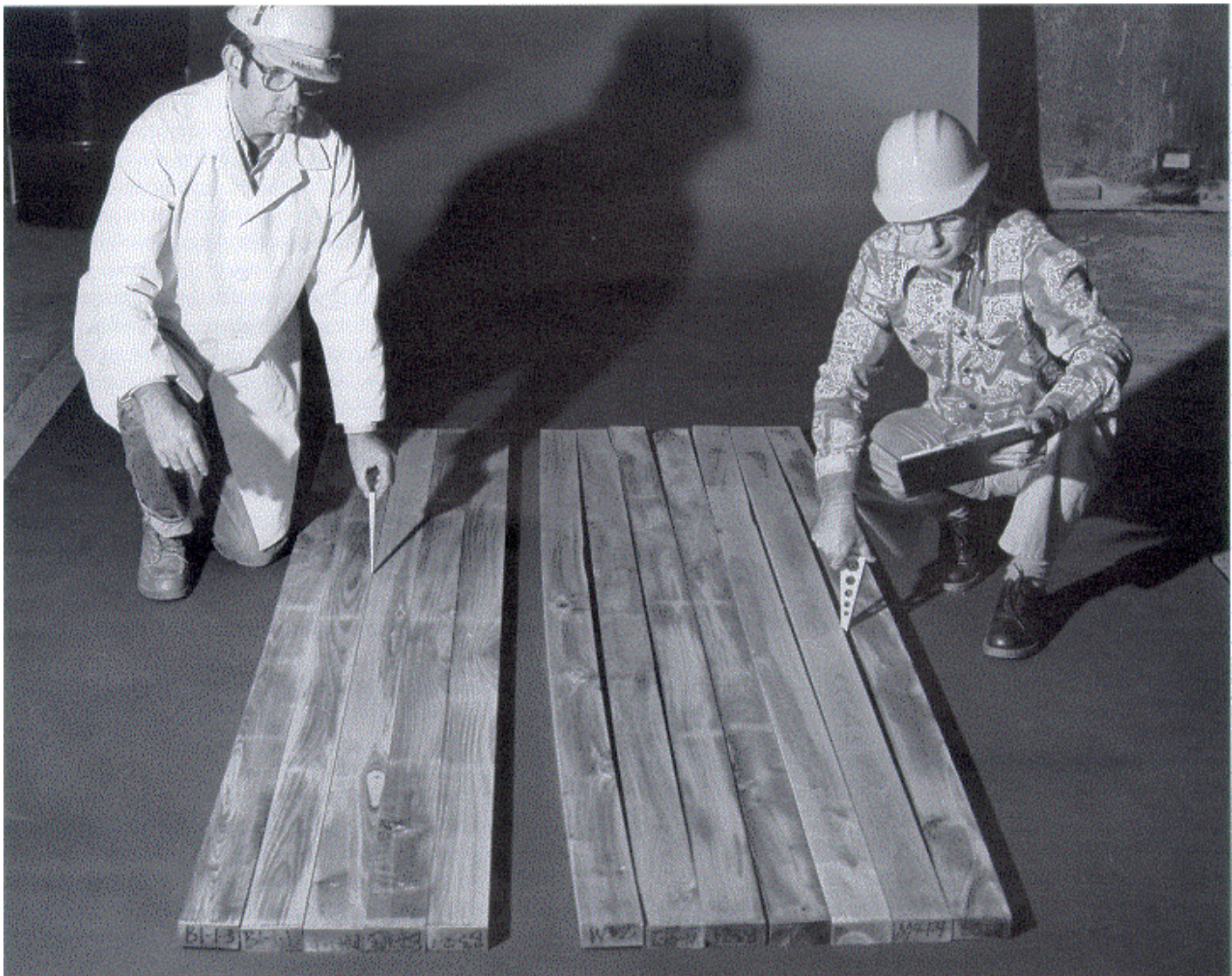
Improved sawmilling and drying techniques developed at FPL allowed significant improvements in the quantity of usable lumber recovered from a log. Here, in 1981, sawing a log in flitches that were subsequently dried then cut into lumber (SDR or saw, dry and rip) reduced the amount of warp that resulted from the drying process.
