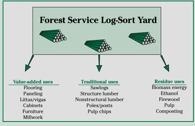
Hierarchy of uses for small-diameter material.
