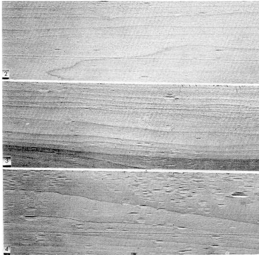
FIGURE 5.—Different degrees of chip marks in yellow-poplar.
