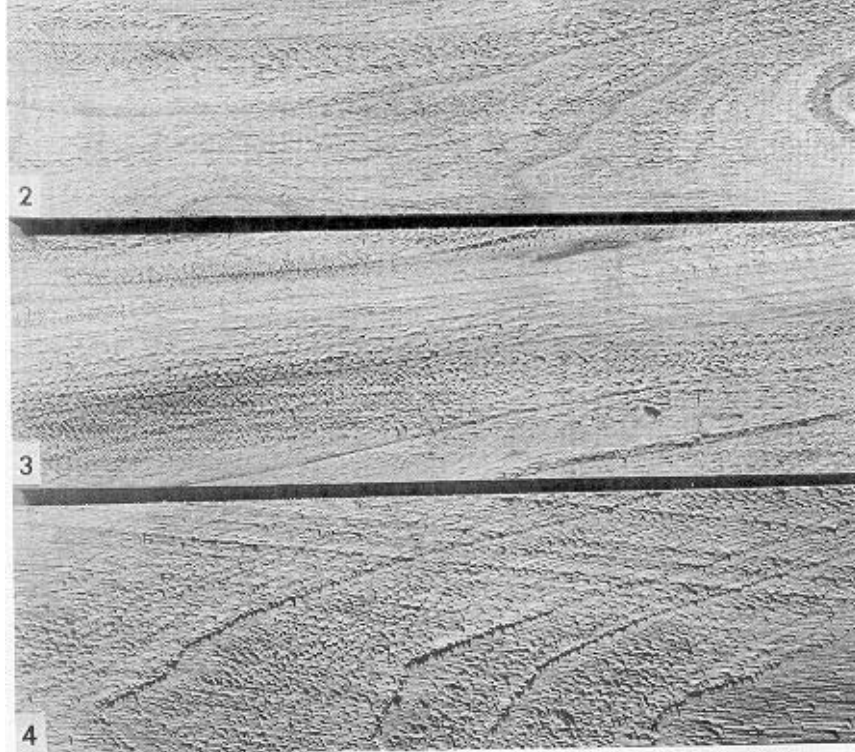
FIGURE 2.—Different degrees of raised grain illustrated by soft elm.
