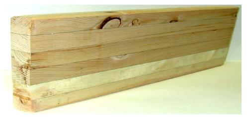
This 1.5- by 9-inch Lam Lumber beam will form the web section of an I-Beam. Laminated flanges will be formed and bonded to the top and bottom of the web. Curved lumber will thus be laminated into a straight beam.
