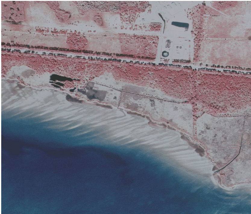
Figure 9. Example of digital orthophotoquad from Apalachicola Bay area, Florida. Color infrared film.
