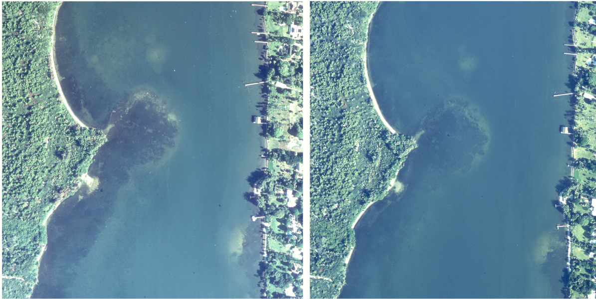
Figure 3. Effect of increased turbidity on ability to resolve SAV bed edges. The right photo was acquired during an algal bloom.
