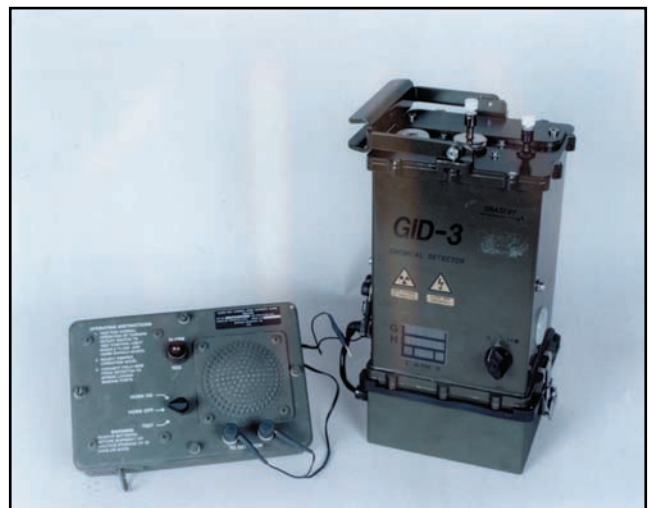
Automatic Chemical Agent Detector/Alarm (ACADA)
