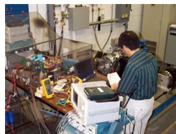
Performance test of DMIC controller driving ORNL's dual stator 20 kW axial gap PM motor
