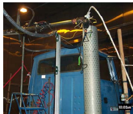
Typical exhaust sampling for truck in Aberdeen environmental chamber.
