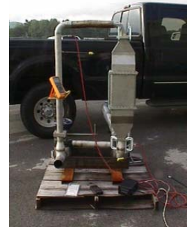
Debugging pleated particulate filter module on Ford F-250 exhaust system
