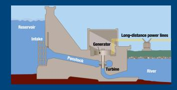
A unique element of the TVA hydropower system is the Raccoon Mountain Pumped Storage Plant, near Chattanooga. The plant consists of two reservoirs, one above the plant at the top of Raccoon Mountain, and the other below it. In periods of low power demand, water is pumped from the lower reservoir to the upper one. Then, when demand is higher, water is released through a tunnel to the powerhouse to generate electricity.
