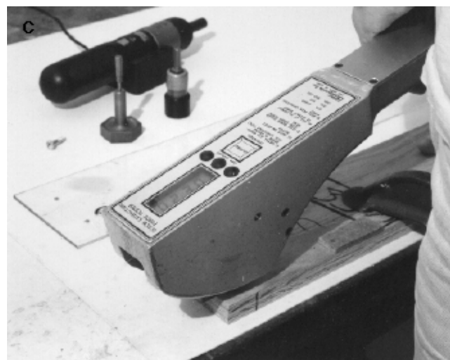
Figure 4—Screw-withdrawal test. Battery-powered screwdriver and jig are used to drill pilot hole (A) and insert screw (B); screw-extraction-force tool is used to withdraw screw while peak withdrawal force is monitored (C).
