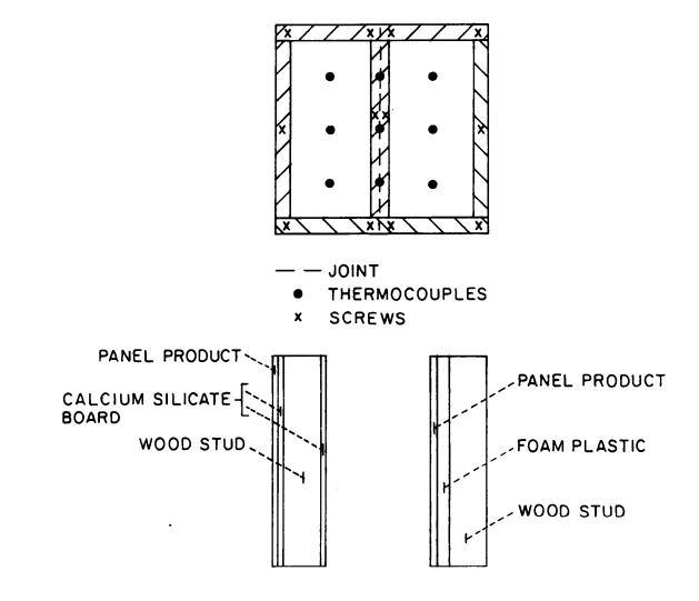
Figure 1.--Diagram of test specimens.
