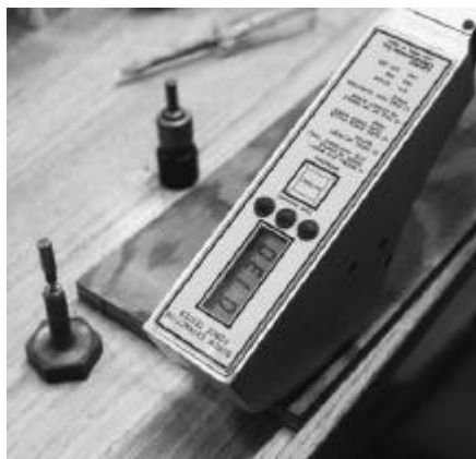
Figure 5. Screw-pull test using hand-held load cell.
