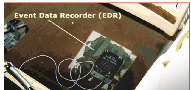
An electronic data recorder, or "black box," installed under the front seat of an automobile collects and stores information about crashes—such as vehicle speed, braking, and passenger seat belt use—that can be used in the investigation of accidents.
