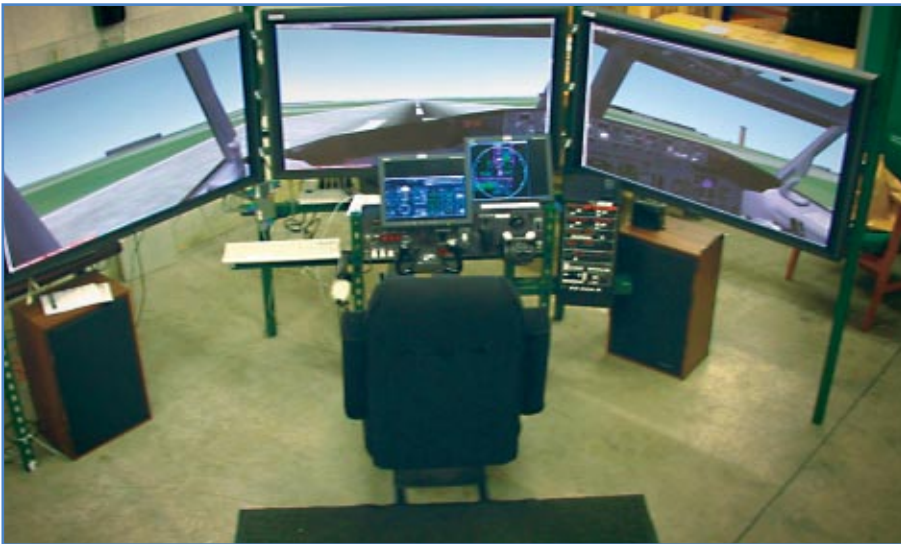
Volpe staff use this general aviation simulator with surface map display in human factors research. The simulator is on loan to the Volpe Center from the FAA’s William J. Hughes Technical Center.
