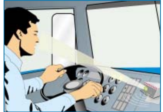
The drowsy driver warning system uses low-level infrared signals (which are not visible) to monitor eye closure.
