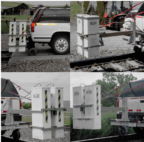
Figure 3. Various GPR configurations on hi-rail vehicles
