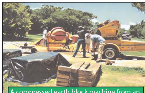
A compressed earth block machine from an Iowa manufacturer will be used to build schools in Kabul, one of them for girls.
