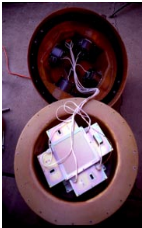
Figure 7. Photo showing the battery compartments inside the Breco Bird Scarer©
