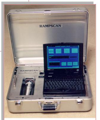
EML RAMPSCAN: A portable, attaché -sized, battery-operated gamma radiation measurement and analysis system used to rapidly assess ("Go"/"No Go") fission product likelihood from freshly collected air filters.
