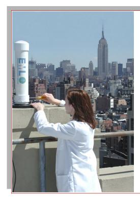
EML Comprehensive Radiation Sensor (CRS): A low cost gamma-ray detector that can easily distinguish anthropogenic fission and activation from natural radiation.
