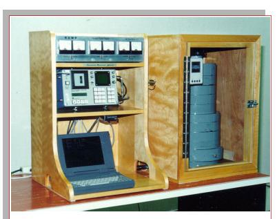
EML RAMS: A particulate collection system with a sodium iodide gamma detector applicable for precise attribution and characterization currenly used in EML's Remote Atmospheric Measurements Program (RAMP).
