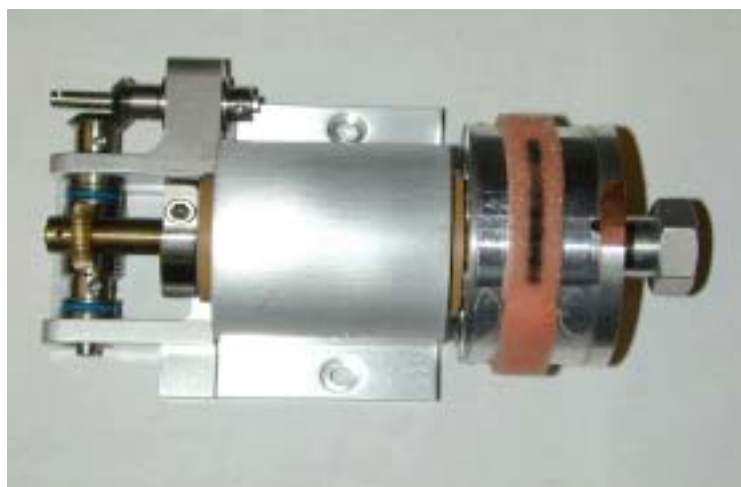
Figure 6. PASS drums, holding the collected aerosols are mounted on a SEM rotation stage control and placed, uncoated, directly in the SEM for analysis.
