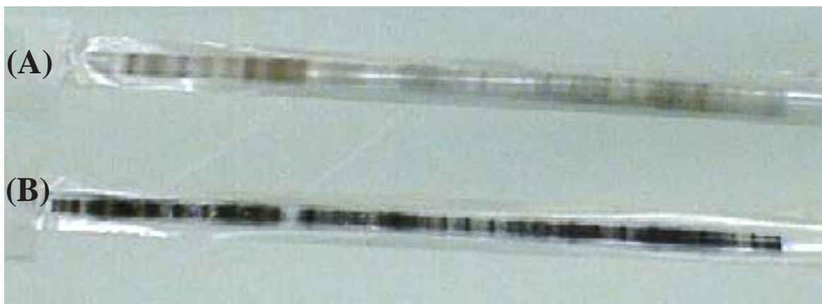
Figure 2. Photograph of 1 month deposit of collected aerosol in two size ranges: (A) coarse particles, 2.5 \mu\text{m} to 10 \mu\text{m} ; and (B) fine particles, 0.3 \mu\text{m} to 2.5 \mu\text{m} .
