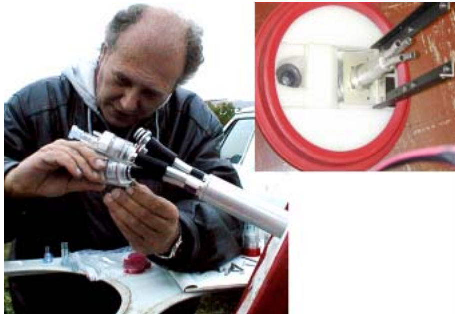
Figure 8. Four separate filters are mounted on the 4-way splitter.
