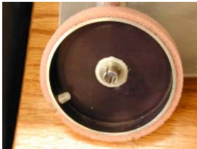
Figure 5. Shown is EML's impactor drum with a PUF ( polyurethane foam) impaction collection surface.
