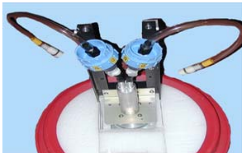
Figure 7. Two independent 47 mm filters are controlled by PASS.
