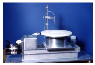
Modular design, assembled with commercially available components, delivers a repeatable amount of liquid to precise locations.
