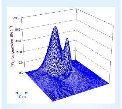
An example of the use of ISDMAP to get a best estimate of the distribution of the contaminant. Mapping of depleted uranium (DU) in soil using data from 19 *in situ* spectrometric measurements and 8 soil samples.
