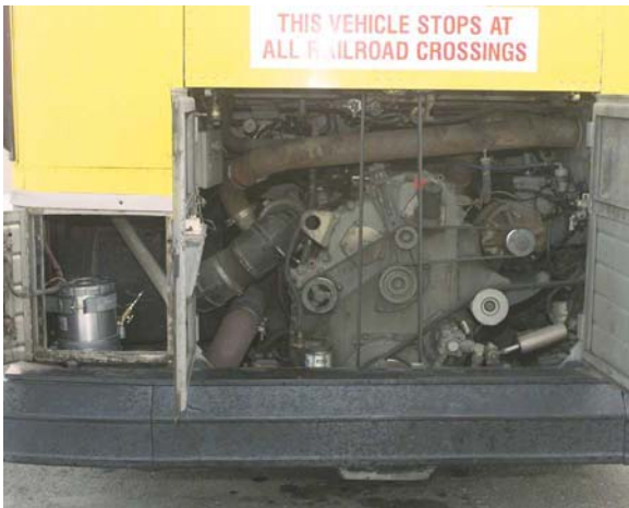
Figure 7. View of engine and filter system on a bus with a Series 50 Detroit Diesel engine.
