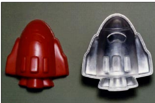
A polyethylene child's toy (left) served as the pattern for this spray-formed, tin-copper alloy die.
