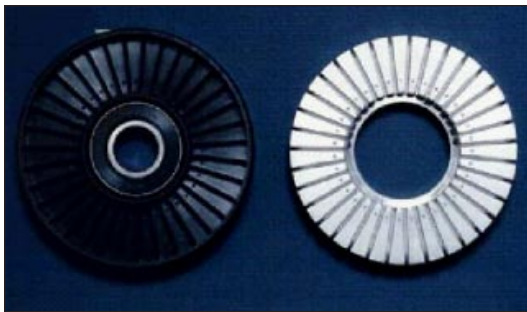
The die (right) was created out of P20 tool steel on a ceramic pattern made from the plastic engine pulley form on the left.
