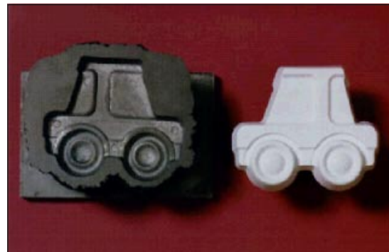
With D2 steel alloy (left), RSP Tooling precisely recreated the raised letters on the ceramic mold (right).
