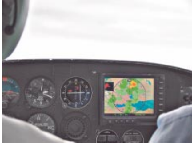
Technology exists to display current weather information graphically to the pilot en route. The challenge is to make the information available to every aircraft throughout the National Airspace System. Photo courtesy FAA Capstone program.
