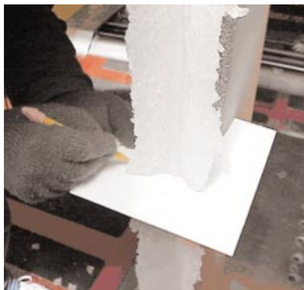
Figure 3-DOD-22. Ice formation from a clustered supercooled water distribution in the NASA Glenn Research Center Icing Research Tunnel. U.S. Army Photo
