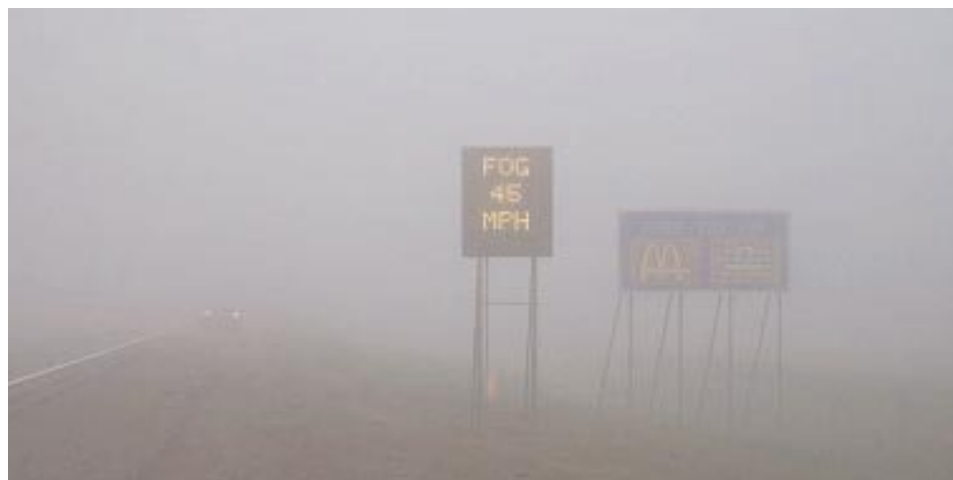
Figure 3-DOT-8. Dynamic message signs enable drivers to take precautionary actions based on weather conditions.
