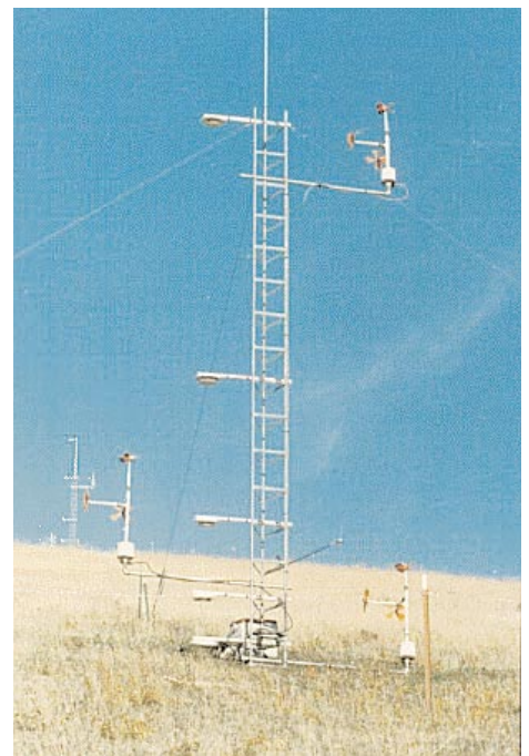
Figure 3-DOE-2. Meteorological towers record temperature and wind direction and speed at various levels.
