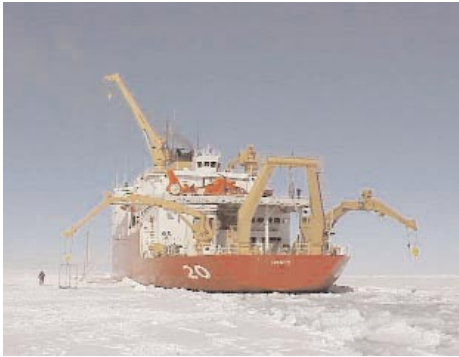
Figure 3-DHS-2. USCGC HEALEY, the Coast Guard's new icebreaking research vessel, conducting ice trials.
