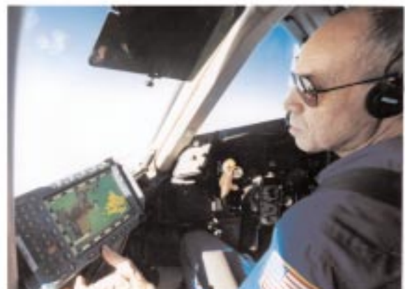
Figure 3-NASA-4. NASA and aviation industry vendors have developed an initial Aviation Weather Information (AWIN) system which is graphical and intuitive for ease of use. Designed to replace bulky, text printouts, AWIN will put graphical weather information in the cockpit.
