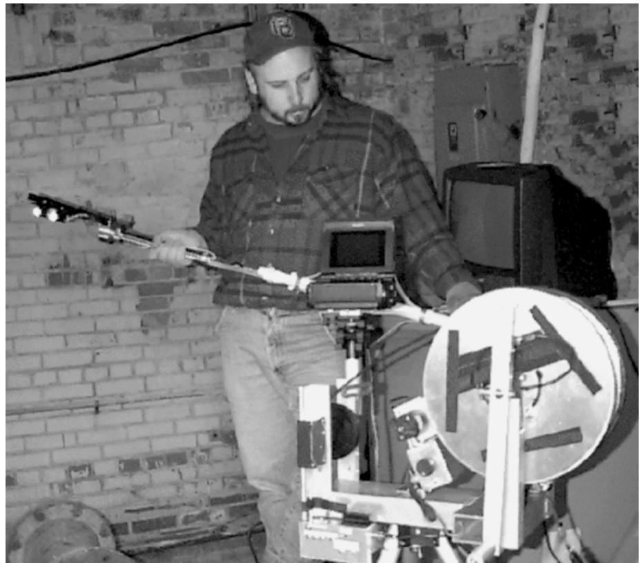
USGS hydrologist Kevin Grazul performing borehole video logging at Philadelphia Naval Complex production wells.
