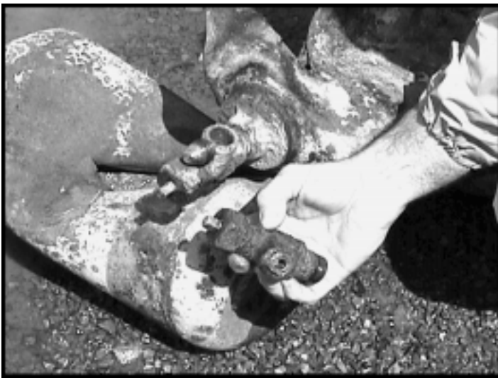
Unearthed ethylene oxide cylinders at NSA Mid-South, showing deteriorated cylinders and valves.
