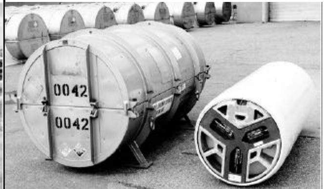
**Figure D-Uranium Hexafluoride (UF<sub>6</sub>) Overpack and Bare 30" Cylinder**
