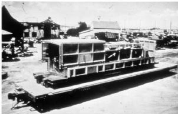
**Figure C-Power Reactor Spent Fuel with Personnel Barrier**
