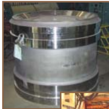
Prototype waste package (top) and the Long-Term Corrosion Test Facility (bottom).
