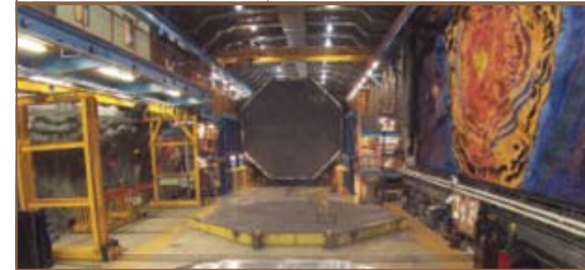
Detector planes for MINOS neutrino detector.
