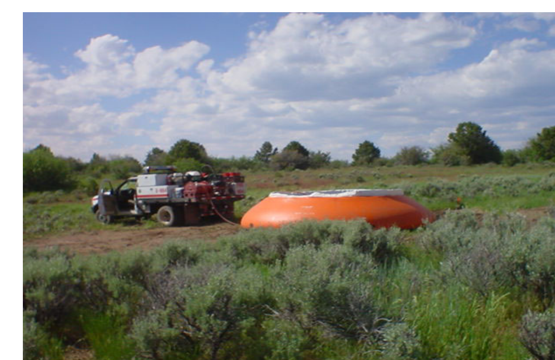
Water tank for structure protection
