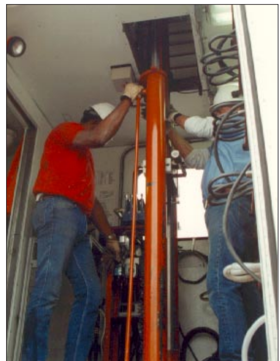
Figure 1. SCAPS with LIF sensors.
