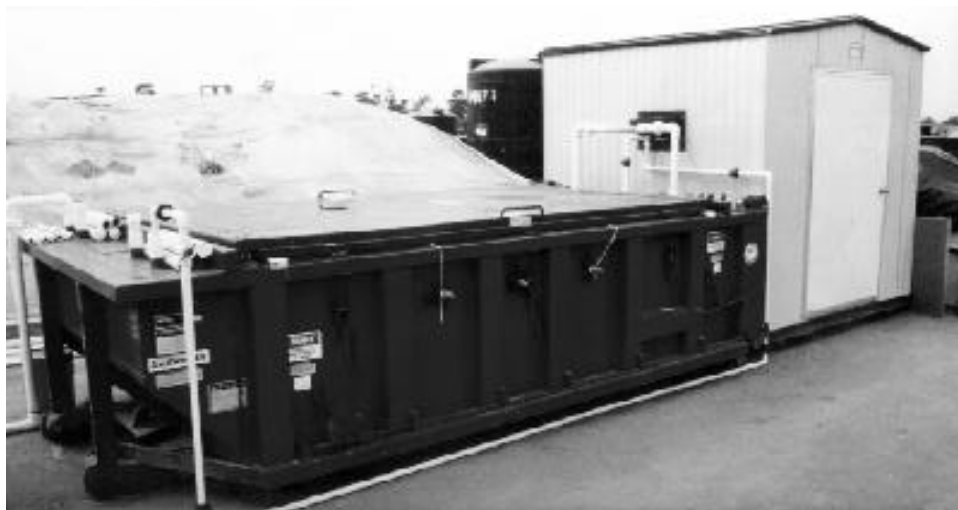
Figure 1-1 Picture of the 10 yd 3 biocell at the National Test Site, Port Hueneme, California.
