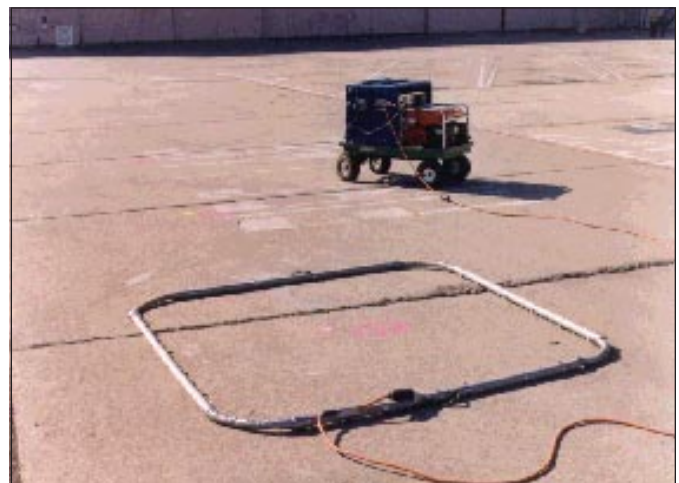
Figure 2. EMR source coil and frequency generator.
