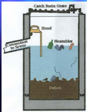
Types of Pollution Found in Catch Drain Basins
