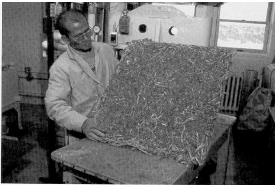
Figure 8.6 A laboratory produced low-density, cement-bonded composite panel. full scale panels such as these are used in construction.
