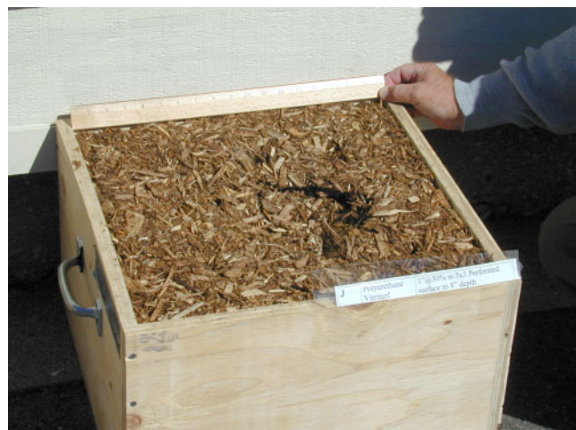
Figure 8—Polyurethane stabilized specimen after three impact events.
