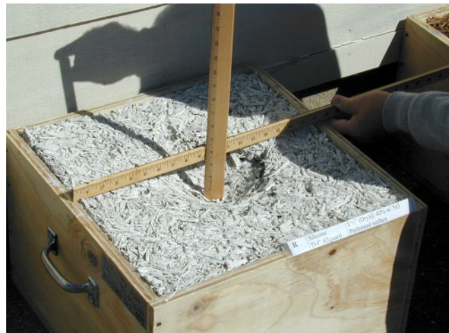
Figure 7—Typical silicone stabilized specimen after three impact events.
