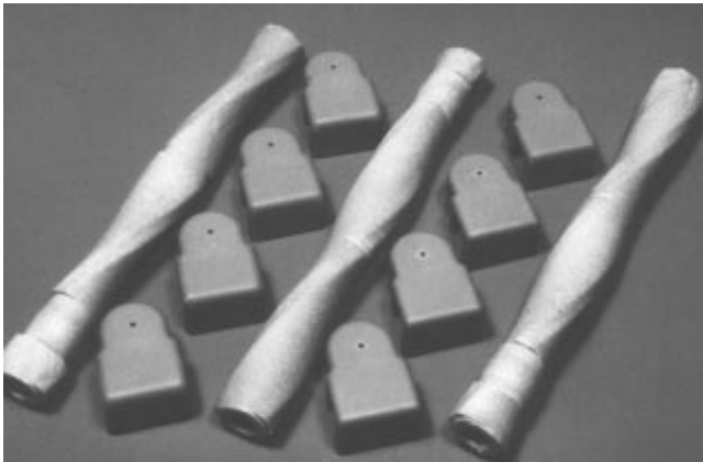
Vacuum cleaner beater bars and battery terminal covers (wood flour/polypropylene).
