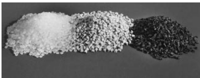
Figure 5—Examples of pelletized thermoplastic feedstock (left to right): virgin unfilled feedstock, feedstock reinforced with waste wood fiber, feedstock reinforced with waste newspaper (ONP) fiber.
