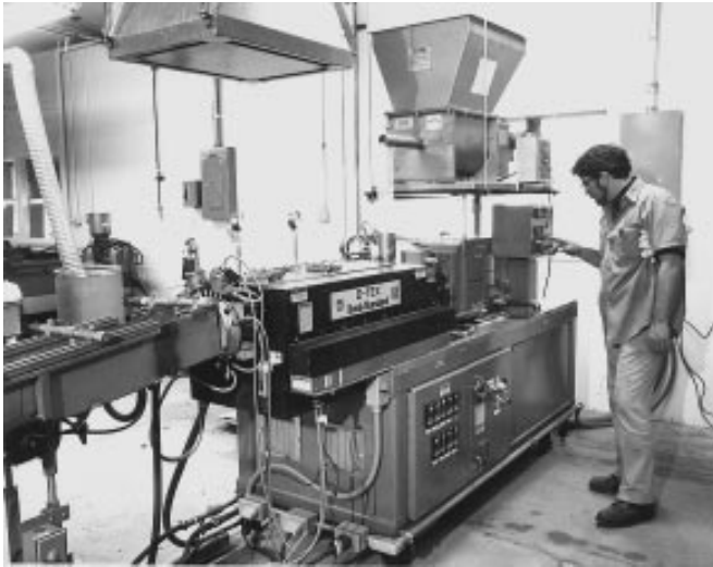
Figure 3—Compounding and pelletizing equipment at FPL.
