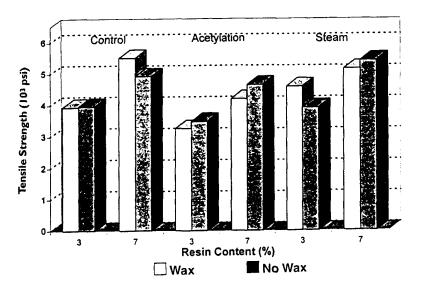
Figure 3. — Effects of treatment, resin content, and wax content on tensile strength parallel to the surface.
