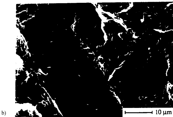
Figure 8 SEM micrograph of fractured specimens. (a) PP/WF composites with EPDM-MA as a impact modifier, and (b) same composite but with MAPP added as a compatibilizer.
