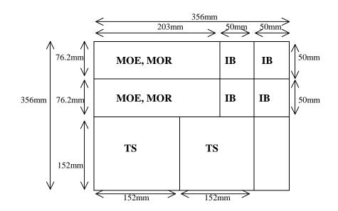
Figure 1. Cutting diagram of PB specimens for testing according to ASTM D 1037-96a. MOE=modulus of elasticity, MOR=modulus of rupture, IB=internal bond, TS=thickness swell. Figure 1 is not drawn to scale.
