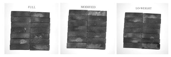
(a) Full-Cell Treatment (b) Modified Full-Cell Treatment (c) Low-weight Treatment
