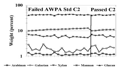
Figure 1. Comparison of chemical composition of 24 randomly selected samples of Southern pine 2x6 lumber of which 17 failed and 7 passed the AWPA Standard C-2 penetration requirement.
