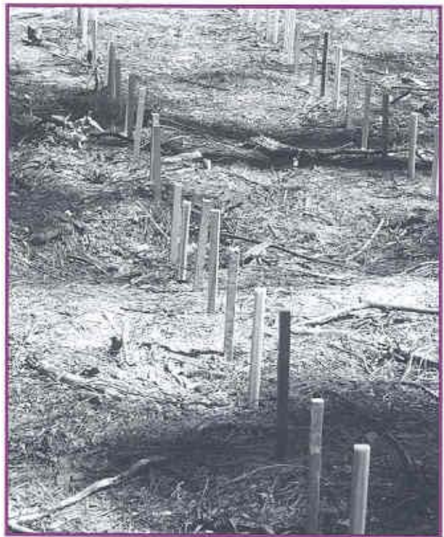
Figure 6a. - In-ground field tests on WPC durability.
