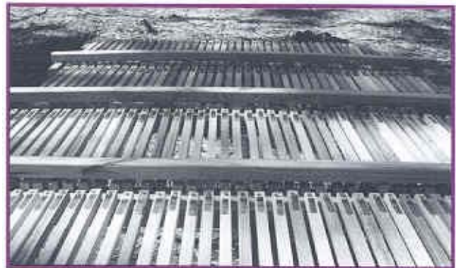
Figure 6b. - Aboveground field tests on WPC durability.
